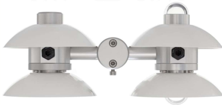
Figure 31. NR01 4-component net radiometer (pyrgeometers on the left and pyranometers on the right of the image).
